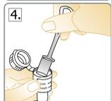
**Stroking of the collector sponge tip can be done in any linear direction, or dabbling, or swirling over the surface. You will inevitably wet the surface with the buffer solution as you are wiping - this is normal. DO NOT DEPRESS THE SPONGE TIP TOO HARD OVER THE SURFACE.**
